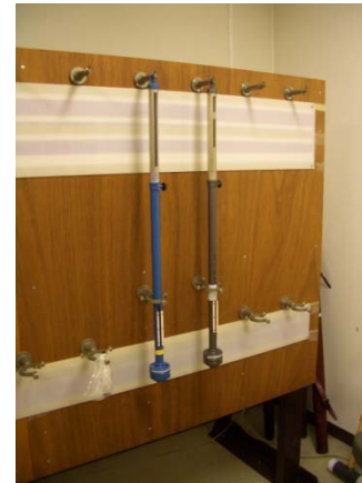
Sub Standard Travelling Kew mercury barometer Serial No 610 /440228 Type 00.06100.100000 No.702055.006 Made in Germany
